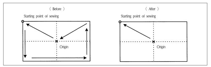
As SPS-1811 machines is equipped with reverse devices, origin search motion is performed as shown in the Before picture and feeds back to the starting point of sewing. However, if there is no reverse device, search motion takes place very slowly. This quick origin search motion function ensures fast origin search as shown in the After picture and feeding back to the starting point of sewing.
