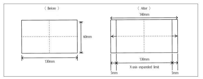
Caution) The sewing limit function is always defaulted at DISABLE and the sewing limit is set at the standard size for each type at the factory.
