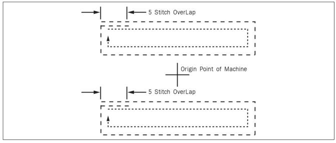
OverLap function can apply to the pattern design of closed roof that start point and end point meet. Except, though it is not closed roof type of pattern and start point and end point have 1mm of distance, OverLap function can use.
