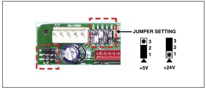
▶ The input power supply to the sensor can be altered to +5V / +24V by changing the BR jumper at the upper left side of the I/O board.
