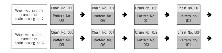
It is used to work with the various patterns randomly. To use the function, the parameter number related to general sewing, "<u>054 Chain No.</u>" should be set to the other numbers except "0". Set the parameter number related to general sewing, "055 Chain Select." to be automatic or manual.
